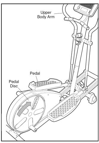
To dismount the elliptical exerciser, allow the pedals to come to a complete stop. The elliptical exerciser does not have a freewheel; the pedals will continue to move until the flywheel stops. When the pedals are stationary, step off the higher pedal first. Then, step off the lower pedal.
